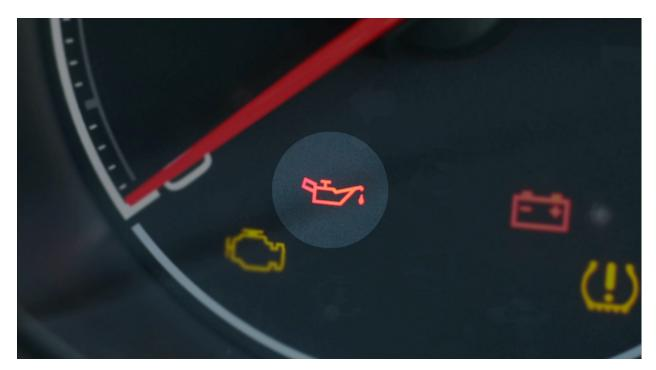
This one—this is the oil light. This is either low oil pressure or low oil levels, and that means that your car is having a heart attack—right now. Pull over. Stop. Don't turn it on until somebody tows you out of there.
